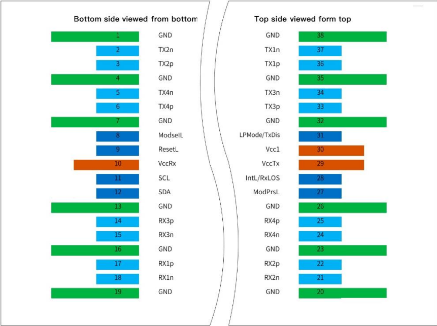
Figure 2 QSFP112 Module contact assignment
