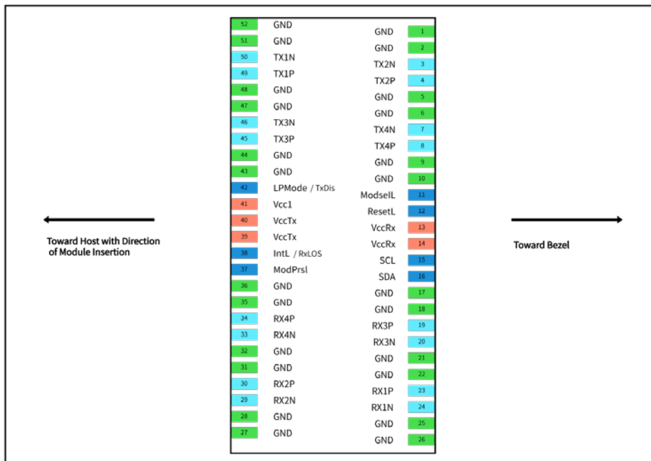
Figure 3 QSFP112 Host PCB pad assignment
